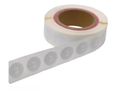
An NTAG DNA C29 tag from NXP can be used to automatically connect to web services, without the need for a dedicated app. Using these tags, together with webbased authentication services, you can now set up AES-128 tag authentication, use three-pass mutual authentication (where only an authorised host can access the tag), and establish a secure channel for data transmission.
